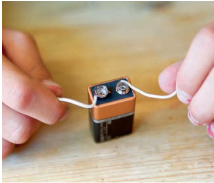
Fig. 3: Attach the wire to the 9-volt battery.
